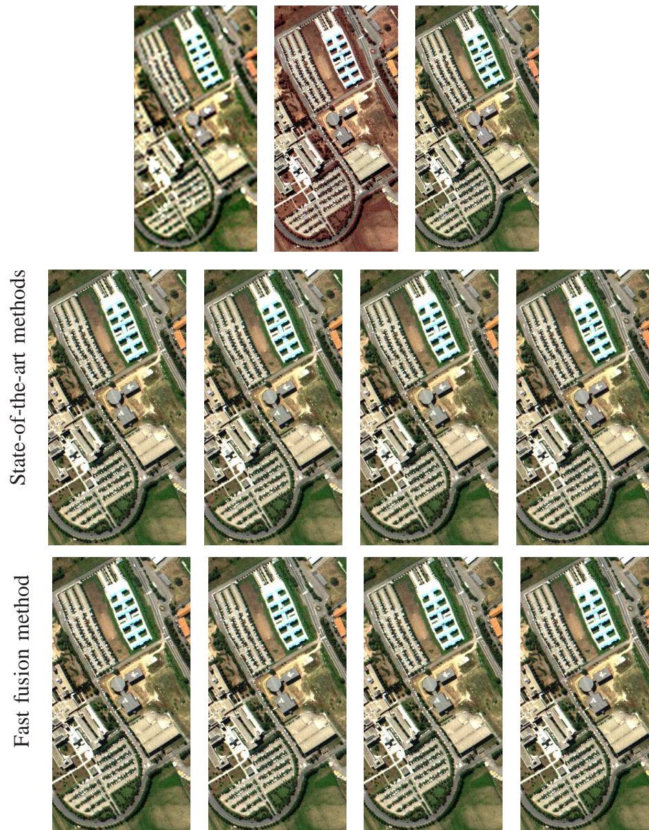
Fig. 1. HS+MS fusion results. Top: HS image (1st column), MS image (2nd column) and reference image (3rd column). Middle and bottom: state-of-the-art-methods and corresponding proposed fast fusion methods, respectively, with various regularizations: supervised naive Gaussian prior (1st column), unsupervised naive Gaussian prior (2nd column), sparse representation (3rd column) and TV (4th column).
