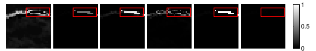
Fig. 4. Map of the re-scaled abundance estimation errors for the third endmember at time t = 2 (from left to right: true abundances, estimation error of VCA/FCLS, SISAL/FCLS, rLMM, OU and the proposed method). Except for the proposed method, the results exhibit notable errors in pixels corrupted by outliers (area in red).
