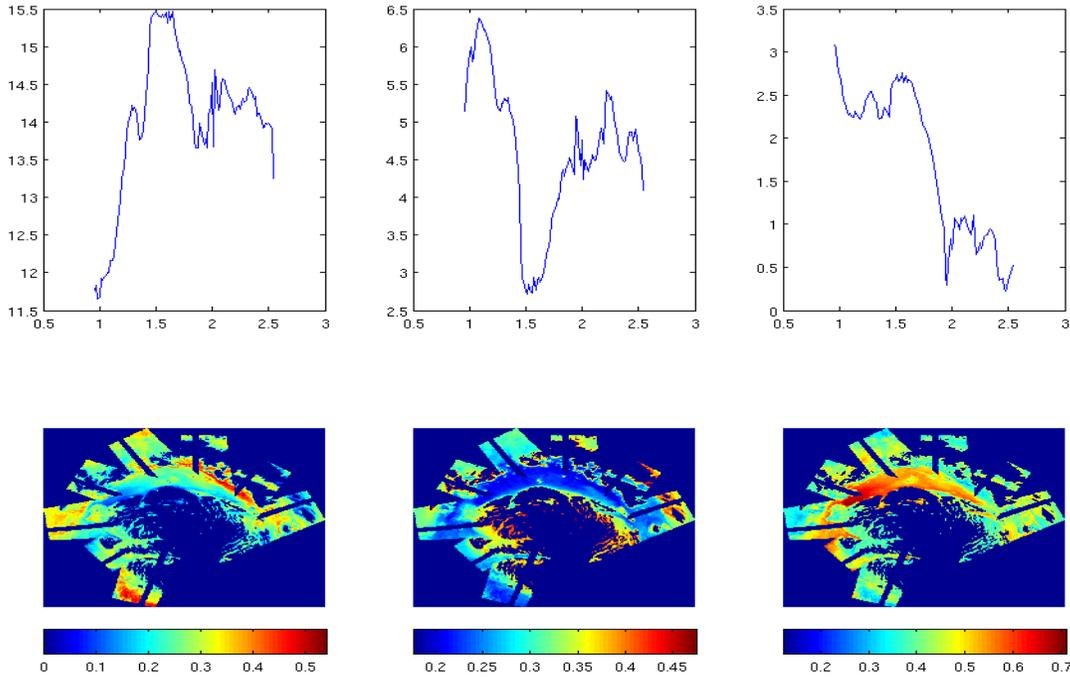
**Fig. 2.** Results of the separation under positivity constraint only (BPSS1): estimated material spectra (top) and corresponding abundance maps (bottom) represented in color from blue (0) to red (maximum).
