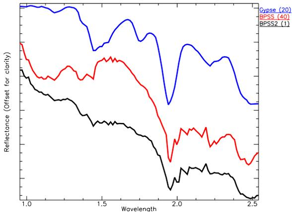
**Fig. 4.** Spectra estimated by the positivity only (BPSS1, red), positivity and additivity (BPSS2, black) and the laboratory spectra of gypsum (blue). For clarity, all spectra have been scaled with a the factor indicated on the legend.
