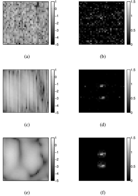
**Fig. 3.** Reconstructed ultrasound image and the magnitude of the reconstructed Fourier domain using: (a) and (b) Bernoulli Gaussian Bayesian approach presented in [8], (c) and (d) reweighted conjugate gradient optimization, (e) and (f) the proposed Bayesian optimization method.
